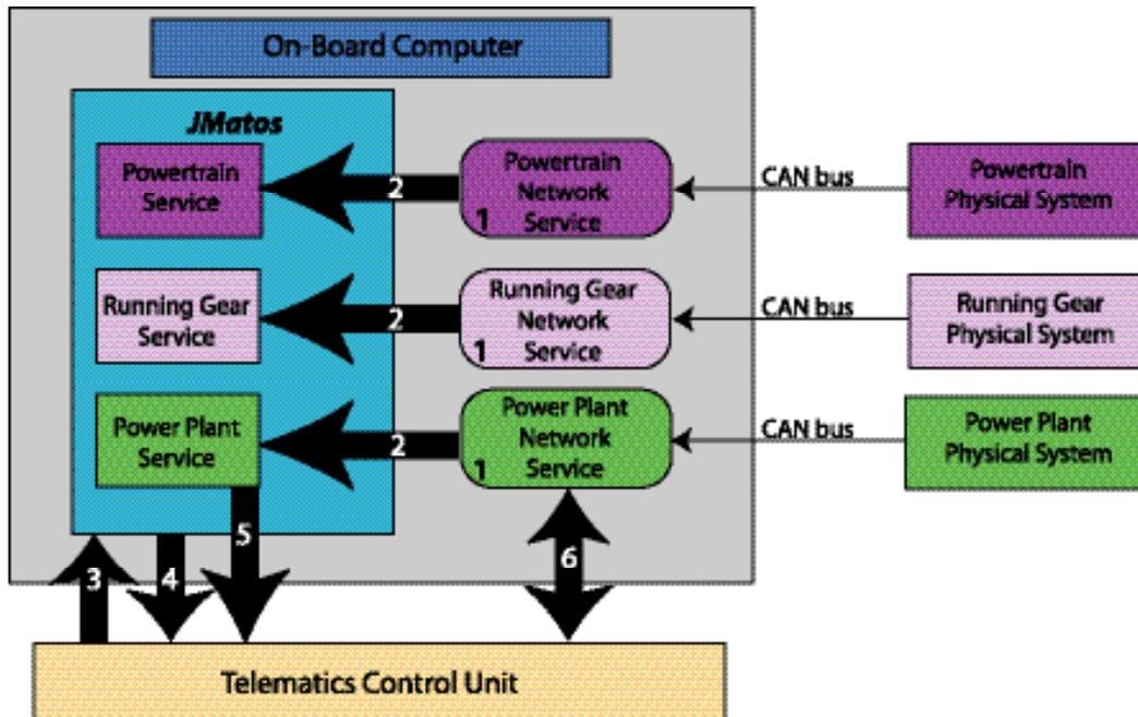
Figure 1: A model for Telematics Control Unit interaction with automotive subsystems using *JMatos*™.
